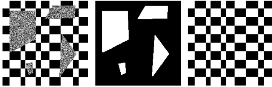
Figure 7.5: Illustration of completing an image as low-rank matrix with some entries masked or corrupted. Left: the masked/corrupted image \mathbf{Y} ; middle: the mask \Omega ; right: the completed image \hat{\mathbf{X}} .
