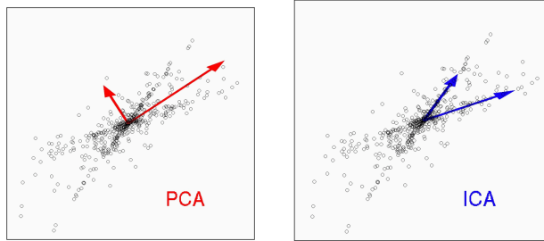
Figure 1.13: PCA (left) versus ICA (right). Note that PCA finds the orthogonal vectors that approximately span the data, while ICA finds (not necessarily orthogonal) vectors that independently combine to approximately form the data, as well as the coefficients of this combination.
